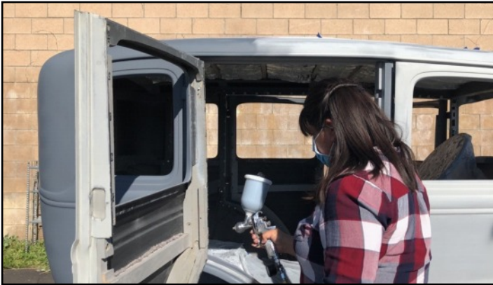
Priming before applying final paint color.
