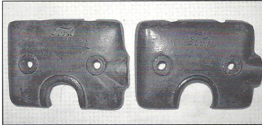
Ford script terminal box covers used from the beginning of production to April 1928. The script location varied.
